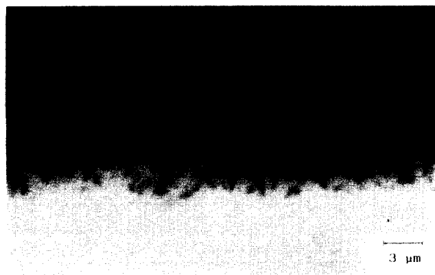
Fig. 2. Oxide scale on preoxidized kovar.
